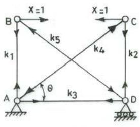
FIG. 17.17. UNIT FORCES ALONG REMOVED MEMBER
