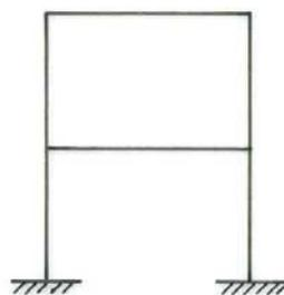
FIG. 5-3. EXTERNALLY AND INTERNALLY INDETERMINATE PLANE SYSTEM
