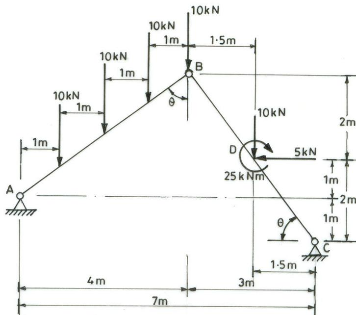
FIG. 8-5. THREE HINGED ARCHED STRUCTURAL SYSTEM AND LOADING.
