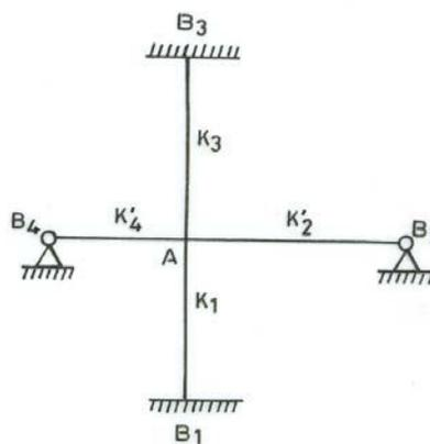
FIG.15-4. PLANE FRAME WITH THREE DEGREES OF FREEDOM
