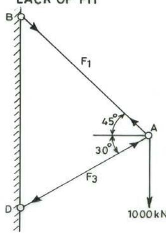
FIG.17-12. DETERMINATE CANTILEVER TRUSS
