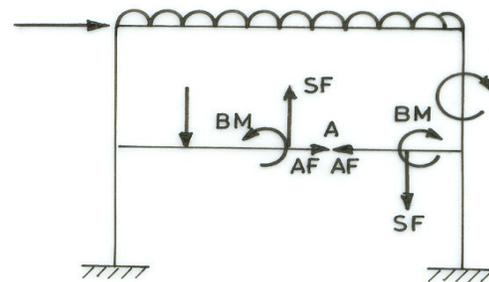
FIG. 2-6. INTERNAL FORCES DEVELOPED AT SECTION A DUE TO APPLIED LOADING.
