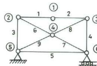
FIG. 9-7. PARTIAL MECHANISM
