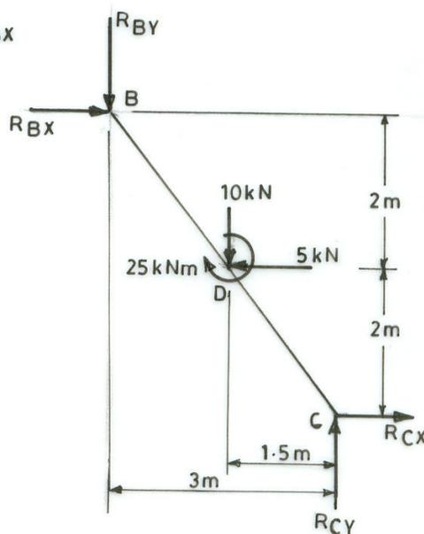
FIG. 8-7. FREE BODY DIAGRAM OF MEMBER BC WITH UNKNOWN FORCES
