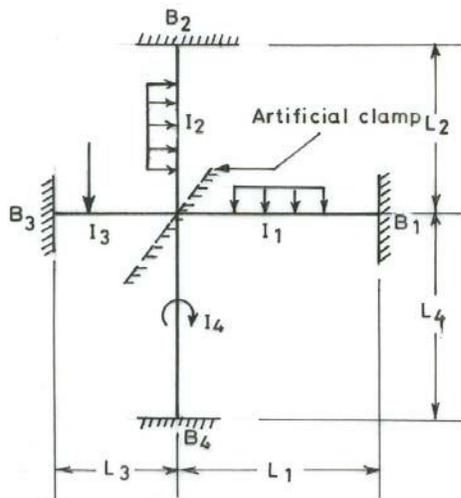
FIG.15-1. PLANE FRAME WITH ONE DEGREE OF FREEDOM
