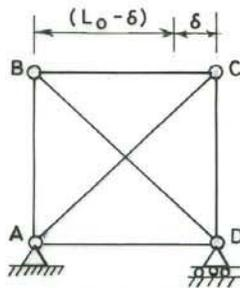
FIG.17-8. TRUSS WITH LACK OF FIT  $\delta$  IN MEMBER BC
