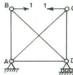
FIG.17-4. UNIT ACTIONS CORRESPONDING TO REMOVED MEMBER
