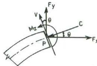
FIG. 10-12. FORCES AT A SECTION OF ARCH
