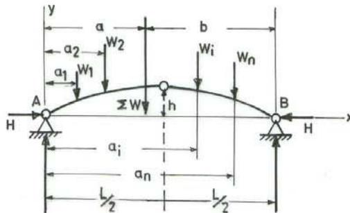
FIG. 10-11. THREE HINGED ARCH UNDER POINT LOADS
