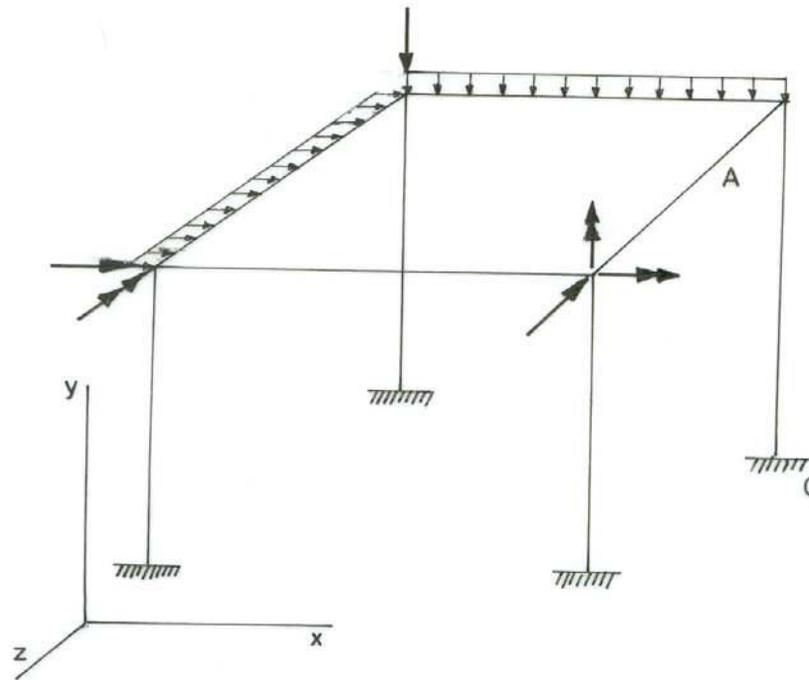
FIG. 2-9. SPACE FRAME SUBJECTED TO GENERAL EXTERNAL LOADING.
