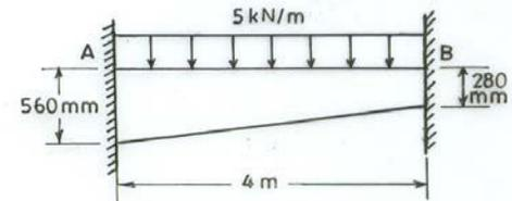
FIG. 14-4. FIXED TAPERED BEAM
