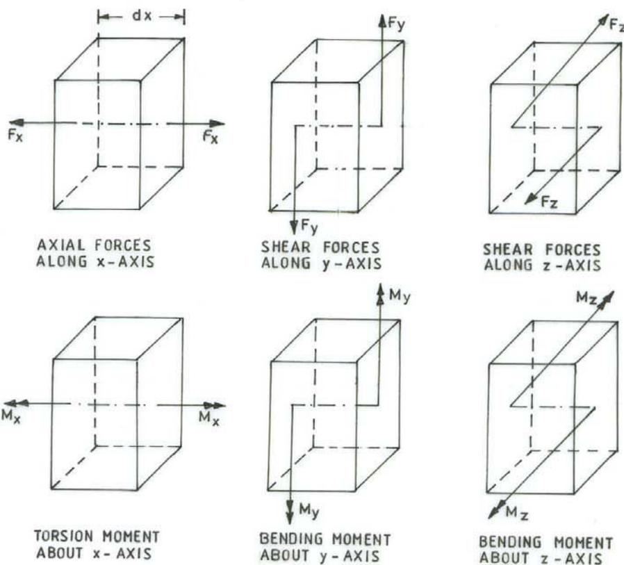
FIG. 3-2. VARIOUS BIATIONS AT A SECTION ON AN ELEMENT
