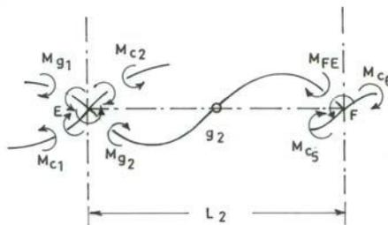
FIG.18-18. FREE BODY DIAGRAM AT NODES OF GIRDER
