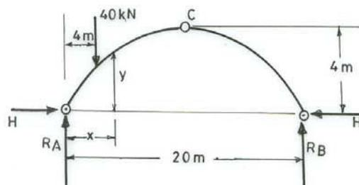
FIG. 10-14. THREE HINGED ARCH UNDER POINT LOAD
