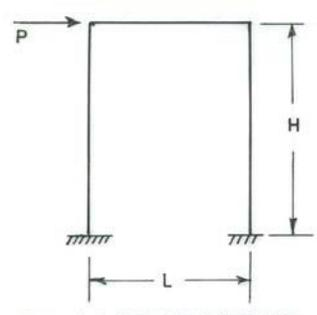
FIG. 18-2. INDETERMINATE PORTAL FRAME
