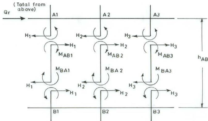
FIG.16-2. FREE BODY DIAGRAM OF COLUMNS OF  $r^{TH}$  STOREY OF FRAME
