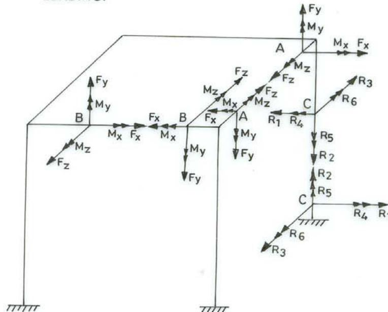
FIG. 2-10. INTERNAL FORCES GENERATED AT A AND B AND REACTIONS DEVELOPED AT C DUE TO EXTERNAL LOADING.
