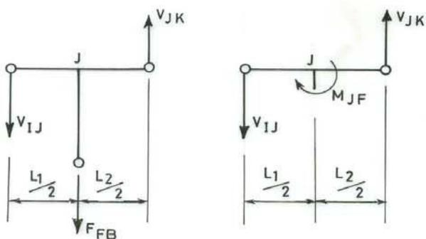
FIG. 18-24. FREE BODY DIAGRAMS FOR COMPUTATION OF COLUMN MOMENTS
