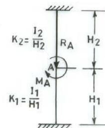
FIG.18-15. FREE BODY DIAGRAM OF COLUMNS AT A
