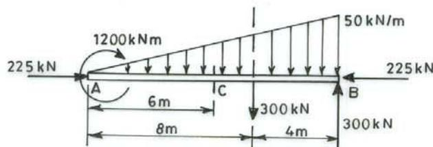
FIG. 8-3. FREE BODY DIAGRAM WITH KNOWN FORCES
