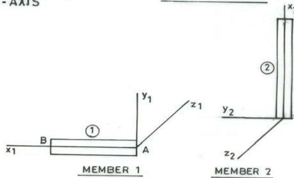
FIG.12-8. GIVEN STRUCTURE AND ITS MEMBERS 1 AND 2
