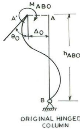
FIG. 16-4. ORIGINAL HINGED AND SUBSTITUTE FIXED COLUMNS
