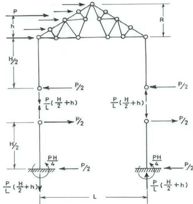
FIG.18-6. DETERMINATE SYSTEM FOR APPROXIMATE ANALYSIS
