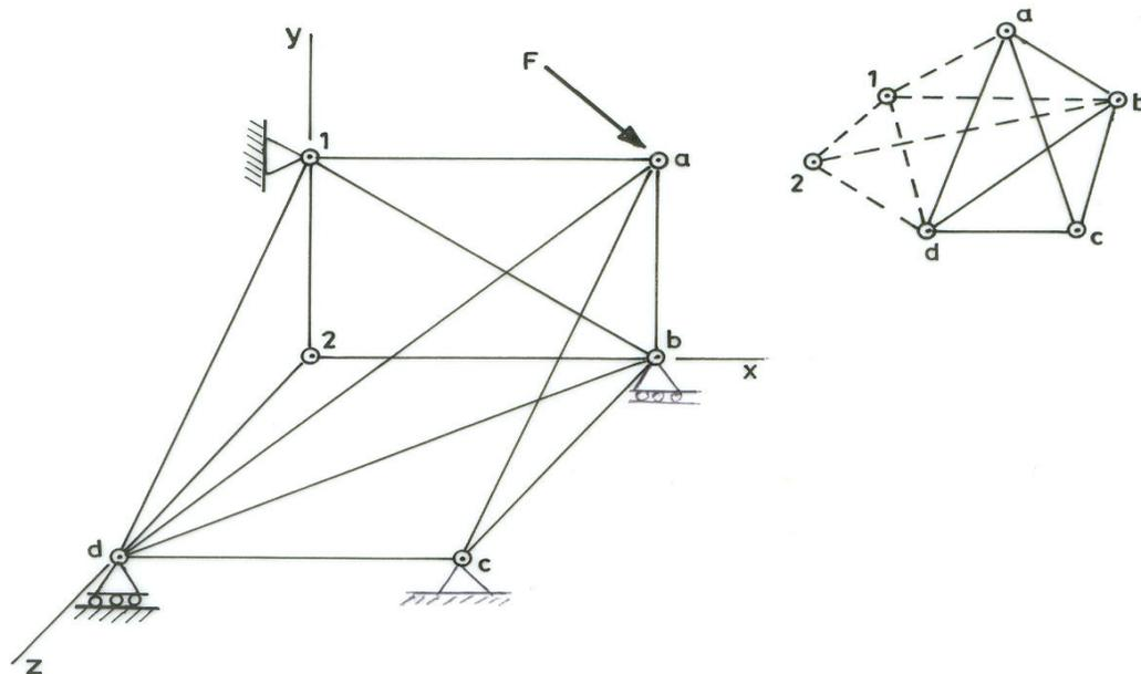
FIG. 2-4. BALL AND SOCKET (UNIVERSAL) JOINTED SPACE TRUSS WITH NODAL LOADING.
