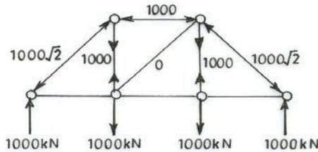
FIG. 9-18. EVALUATED FORCES AND REACTIONS FOR TRUSS
