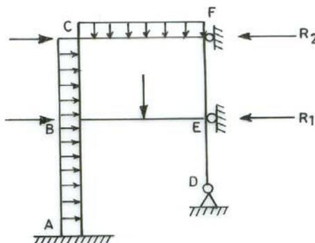
FIG.15-7. GIVEN STRUCTURE WITH TWO CONSTRAINTS AND LOADS
