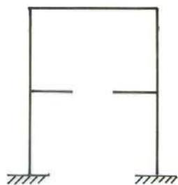
FIG. 5-1. EXTERNALLY INDETERMINATE BUT INTERNALLY DETERMINATE PLANE SYSTEM
