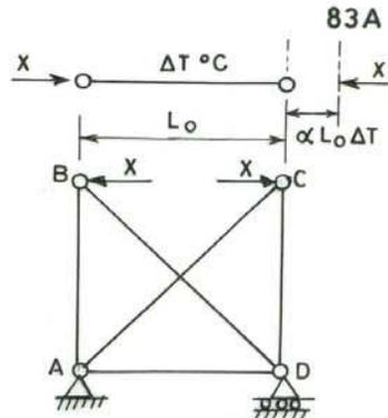
FIG.17-10. DETERMINATE TRUSS BY REMOVAL OF MEMBER SUBJECTED TO TEMPERATURE RISE
