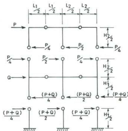
FIG. 18-17. FREE BODY DIAGRAMS FOR APPROXIMATE ANALYSIS FOR HORIZONTAL LOADS
