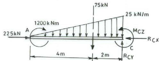
FIG. 8-4. FREE BODY DIAGRAM WITH UNKNOWN FORCES
