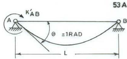
FIG. 13-12. MODIFIED ROTATIONAL STIFFNESS OF MEMBER
