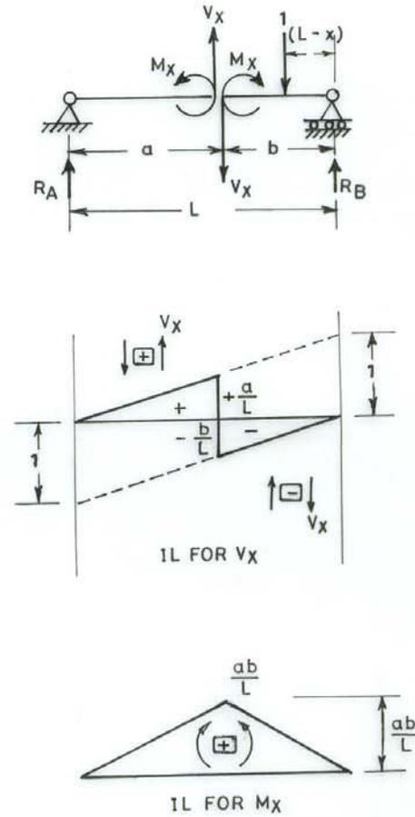
FIG. 11-3. IL FOR INTERNAL FORCES AT A SECTION
