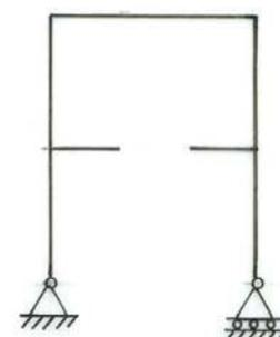
FIG. 5-4. EXTERNALLY AND INTERNALLY DETERMINATE PLANE SYSTEM
