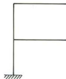
FIG. 5-2. EXTERNALLY DETERMINATE BUT INTERNALLY INDETERMINATE PLANE SYSTEM
