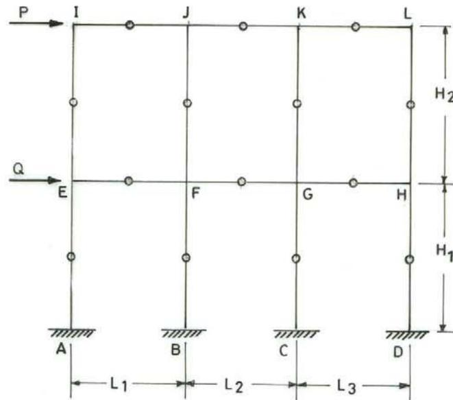
FIG.18-20. INDETERMINATE PLANE FRAME WITH HINGES AT MID POINTS OF ALL MEMBERS
