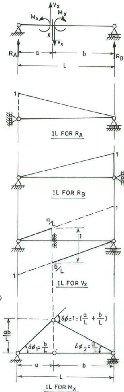
FIG. 11-5. IL FOR INTERNAL FORCES BY MULLER-BRESLAU'S PRINCIPLE
