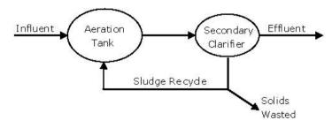
50. The food-to-biomass (F/M) ratio (in kg BOD per kg biomass per day) for the aeration tank is
