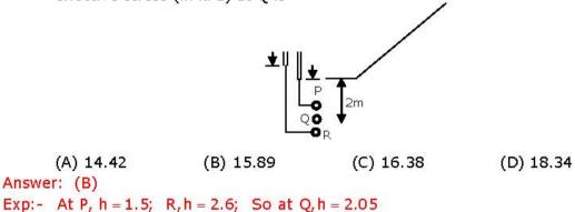
So, effective stress at  $\theta = \sigma^1 = \sigma - \upsilon = Y_{sat} \times H - Y_{sat} \times h$  $= 18 \times 2 - 9.81 \times 2.05 = 15.89$  kN/m<sup>2</sup>
