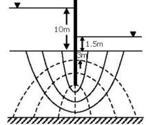
48. The seepage loss (in m<sup>3</sup> per day per unit length of the wall) of water is
