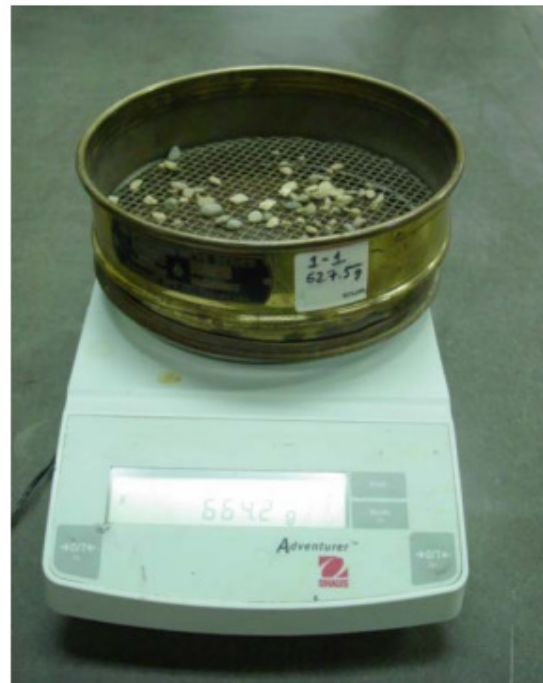
FIG 4.1-PROCEDURE OF SIEVE ANALYSIS.
