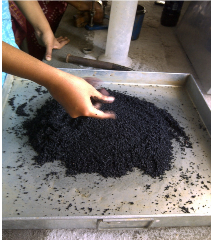
FIG 5.3- MIXING COPPER SLAG WITH WATER.
