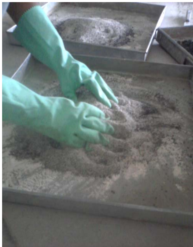
Fig 6.2 mixing of copper slag
