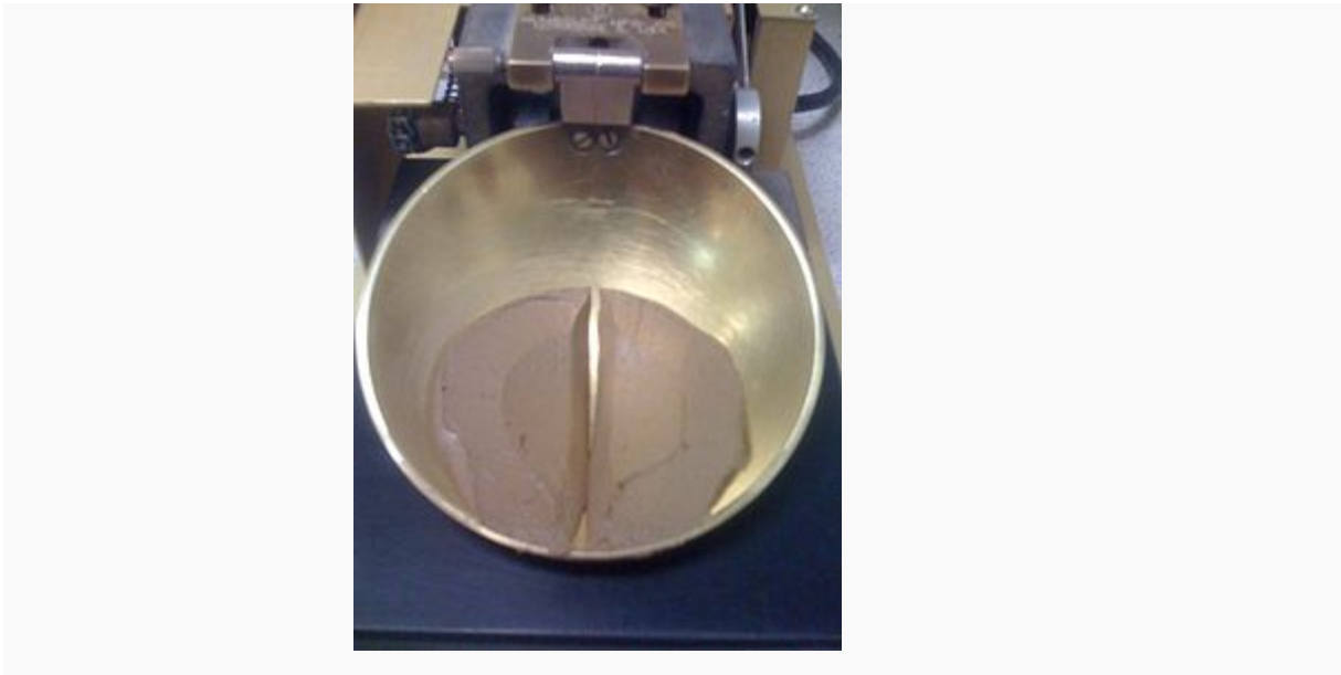
Fig 5.10 Casagrande cup in action
