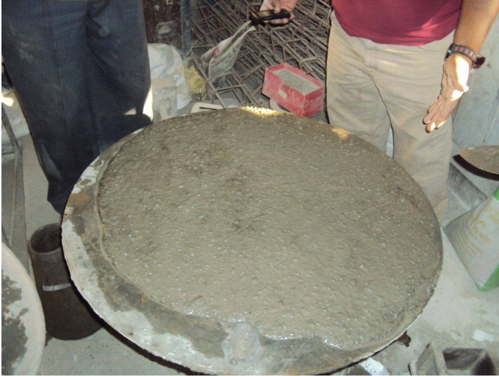
Fig. 3.1 Slump flow test and T_{50\text{cm}} test procedure (SCC mixes)
