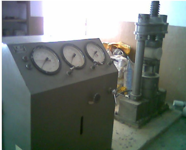
Fig.3.10 split tensile strength test
