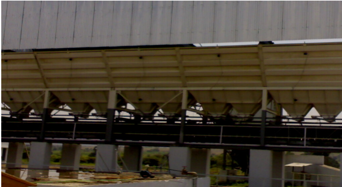
Skip Bucket (Weighing belt)
