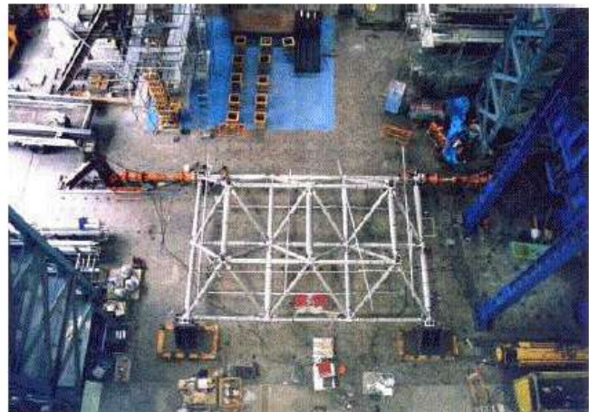
In-plane loading test
