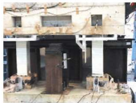
(a) reinforced concrete column (b) SRF columns Photo 2 reinforced concrete column and SRF column after the shaking table test
