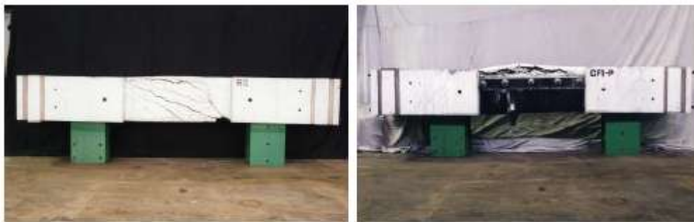
(a) unretrofit beam (b) retrofit beam Photo 1 Specimens during and after tests
