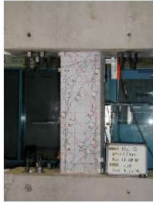
RC SRF (a) Ultimate state (80% of maximum load)
