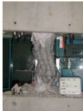
RC (loss of longitudinal stiffness) SRF (b) After test
