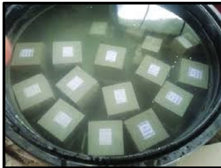
Figure 5: Curing of concrete
